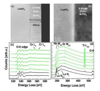
FIG. 2. (Color online) (a) Cross sectional TEM image at large length scale of the 2%Cr, 0.5%Nb doped STO film grown on LaAlO<sub>3</sub> (001) substrate. (b) High resolution TEM image for the interface between the film and substrate. [(c) and (d)] EELS line scans across the cross section of the sample.
