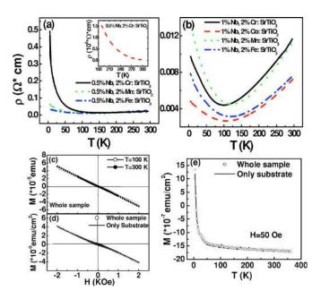
FIG. 3. (Color online) [(a) and (b)] Temperature dependence of resistivity for these thin films: 2%MTE, 0.5%Nb doped STO and 2%MTE, 1%Nb doped STO, respectively. (c)Typical M vs H for one thin film (including substrate) at 300 and 100 K. (d) Comparison of M-H for one sample with a heated pure substrate at 15 K. (substrate area unity: emu/cm<sup>2</sup>). (e) Comparison of M-T for one sample with a heated pure substrate at an applied field of 50 Oe.
