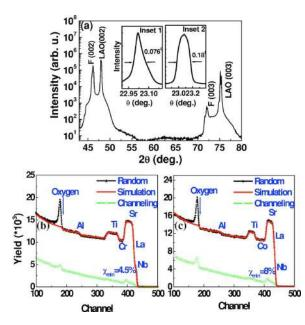
FIG. 1. (Color online) (a) A typical  $\theta$ -2 $\theta$  XRD pattern for 2%MTE, Nb:STO thin films on LaAlO<sub>3</sub> (001). Peaks labeled "F" correspond to the film. Inset 1 shows the XRD rocking curve for a thin film with chromium doping. Inset 2 shows the rocking curve for a cobalt doped one. [(b) and (c)] 3.05 MeV He<sup>+</sup> Rutherford backscattering (RBS) random simulation and channeling spectra for the 2%Cr, 0.5%Nb doped STO and 2%Co, 0.5%Nb doped STO thin films, respectively.
