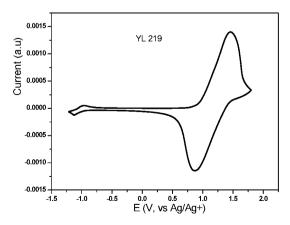
Fig. 3 The first cyclic voltammogram (CV) redox cycle of a PDBF-*co*-TT thin film.
