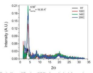
**Fig. 4** X-ray diffraction (XRD) data obtained from spin-coated PDBF-*co*-TT thin films ( $\sim$ 35 nm) on OTS treated SiO<sub>2</sub>/Si substrates annealed at different temperatures.
