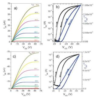
**Fig. 6** The output (left:  $V_{\rm G} = 0$  V to -70 V) and transfer (right:  $V_{\rm DS} = -70$  V) characteristics of an OTFT device with PDBF-*co*-TT thin films without annealing (a and b) and annealed at 100 °C for 15 min (c and d). Device dimensions: channel length (L) = 100 µm; channel width (W) = 1 mm.
