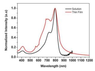
**Fig. 2** UV-vis-NIR absorption spectra of PDBF-*co*-TT in CHCl<sub>3</sub> solution (black) and in thin film (red) on a glass substrate.
