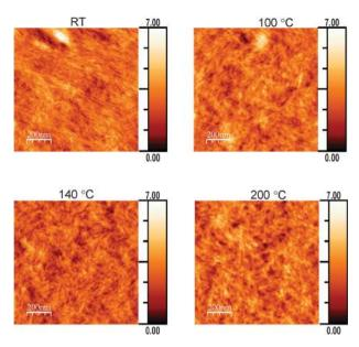
Fig. 5 Atomic Force Microscopy (AFM) data obtained from spin-coated PDBF-*co*-TT thin films (~35 nm) on OTS treated SiO<sub>2</sub>/Si substrates annealed at different temperatures.
