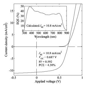
Fig. 8 Current density–voltage curves of the best PDBF-co-TT:PC<sub>71</sub>BM-based solar cell under dark and simulated AM1.5 solar illumination conditions. The inset is the external quantum efficiency (EQE) spectrum under low light levels.
