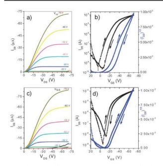
**Fig. 7** The output (left:  $V_{\rm G} = 0$  V to -70 V) and transfer (right:  $V_{\rm DS} = -70$  V) characteristics of an OTFT device with PDBF-*co*-TT thin films annealed at 140 °C (a and b) and 200 °C for 15 min (c and d). Device dimensions: channel length (L) = 100 µm; channel width (W) = 1 mm.
