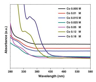
**Fig. 4** Absorption spectra of Zn<sub>0.9</sub>Cd<sub>0.1</sub>S: yCo (0.005, 0.01, 0.015, 0.025, 0.05, 0.12 and 0.18 M) nanoparticles
