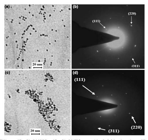
Fig. 3 (a, c) TEM images of  $Zn_{0.9}Cd_{0.1}S:0.0202Co$  and  $Zn_{0.9}Cd_{0.1}S:0.078Co$  nanoparticles. (b, d) Selected area electron diffraction patterns of  $Zn_{0.9}Cd_{0.1}S:0.0202Co$  and  $Zn_{0.9}Cd_{0.1}S:0.078Co$  nanoparticles
