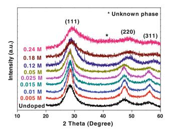
**Fig. 1** X-ray diffraction patterns of Zn<sub>0.9</sub>Cd<sub>0.1</sub>S: yCo (undoped, 0.005, 0.01, 0.015, 0.025, 0.05, 0.12, 0.18 and 0.24 M) nanoparticles
