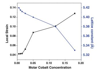
**Fig. 2** Variation in local strain and lattice constant with cobalt concentration in  $Zn_{0.9}Cd_{0.1}S$ : yCo (0.005, 0.01, 0.015, 0.025, 0.05, 0.12 and 0.18 M) nanoparticles
