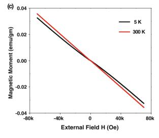
Fig. 6 Magnetization versus applied magnetic field measured at 5, 50, 100 and 300 K. a 0.05 M cobalt concentration, b 0.18 M cobalt concentration, c Magnetization versus applied magnetic field for undoped sample at 5 and 300 K
