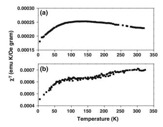
Fig. 8 Variation of  $\chi T$  with temperature. a 0.05 M cobalt concentration, b 0.18 M cobalt concentration
