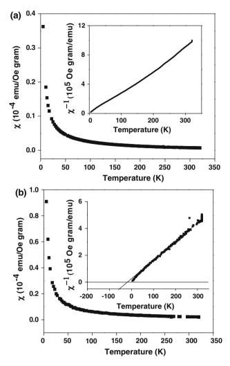
**Fig. 7** Temperature-dependent magnetic mass susceptibility measured under a magnetic field of 500 Oe. *Inset*: inverse susceptibility as a function of temperature: **a** 0.05 M cobalt concentration, **b** 0.18 M cobalt concentration
