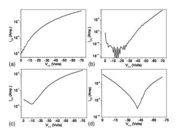
FIG. 5. Transfer characteristic of CuPc based transistors (L:100  $\mu$ m; W: 3 mm) having injecting contact metal (a). Au and (b) Al on SiO<sub>2</sub> gate dielectric, and (c). Au and (d). Al on PMMA/SiO<sub>2</sub> gate dielectric.
