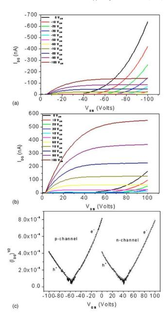
FIG. 2. (Color online) Current-voltage characteristics, (a).  $I_{DS}$ - $V_{DS}$  (*p*-channel), (b).  $I_{DS}$ - $V_{DS}$  (*n*-channel), and (c).  $I_{DS}$ - $V_{GS}$ , of F<sub>4</sub>CuPc based OTFT (L:50  $\mu$ m; W: 3 mm) on SiO<sub>2</sub>/PMMA gate dielectric.
