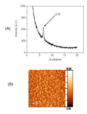
FIG. 6. (Color online) (a) X-ray diffraction pattern and (b) AFM image of  $F_4$ CuPc thin film deposited at room temperature on Si/SiO<sub>2</sub> substrate.
