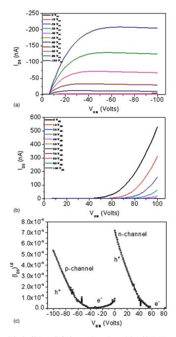
FIG. 3. (Color online) Current-voltage characteristics. (a)  $I_{DS}$ - $V_{DS}$  (*p*-channel), (b)  $I_{DS}$ - $V_{DS}$  (*n*-channel), and (c)  $I_{DS}$ - $V_{GS}$ , of F<sub>4</sub>CuPc based OTFT (L:50  $\mu$ m; W: 3 mm) on SiO<sub>2</sub> gate dielectric.
