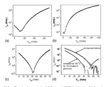
FIG. 4. Transfer characteristic of CuPc based OTFT (L:100  $\mu$ m; W: 3 mm) on PMMA/SiO<sub>2</sub> gate dielectric (a) before and (b) after air exposure measured in glove box under N<sub>2</sub>. (c) and (d) shows transfer characteristic of F<sub>4</sub>CuPc based devices before, and after air exposure, respectively. Annealing of air exposed devices at 100 °C (15 min) in the N<sub>2</sub> filled glove box results in significant recovery of electron transport shown in (d).
