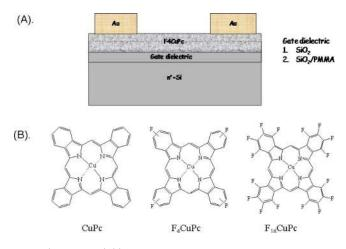
FIG. 1. (Color online) (a) Schematic structure of top contact OTFT used in study, (b) Molecular structure of CuPc,  $F_4$ CuPc, and  $F_{16}$ CuPc molecules.
