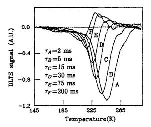
Figure 1. DLTS spectra of Si irradiated with  $Ar^+$  at dose  $1 \times 10^{14} cm^{-2}$  showing negative peak for slower rate windows.
