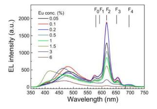
FIG. 1. (Color online) EL spectrum of Eu-implanted MOS devices annealed with RTA at 1000 °C for various Eu concentrations and under an injection current of 5  $\mu$ A. The black solid lines indicate the position of the  ${}^{5}D_{0}{}^{-7}F_{J}$  lines ( $0 \le J \le 4$ ) according to Ref. 10.
