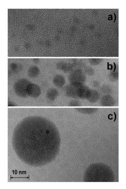
FIG. 3. Bright field cross section TEM images showing Eu/Eu oxide clusters in the SiO<sub>2</sub> layer for 1.5% Eu and annealed at 1000 °C by FLA (a), RTA (b), and FA (c). All images have the same magnification.
