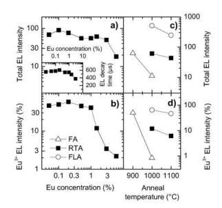
FIG. 2. The dependence of the total EL intensity [(a) and (c)] and the relative intensity of the Eu<sup>3+</sup> emission in percent [(b) and (d)] of MOS structures on Eu concentrations [(a) and (b)] for RTA at 1000 °C and on annealing [(c) and (d)] for an Eu concentration of 1.5%. The inset shows the EL decay time of the  ${}^{5}D_{0}{}^{-7}F_{2}$  line for RTA at 1000 °C.
