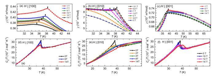
FIG. 6. (a)–(c) Temperature dependence of the magnetic susceptibility at different magnetic fields applied along the *a*, *b*, and *c* directions, respectively. (d)–(f) Temperature dependence of  $C_p/T$  at different magnetic fields applied along the *a*, *b* and *c* directions, respectively.
