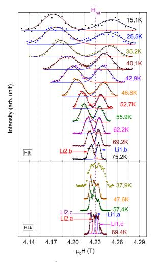
FIG. 8. Field-sweep <sup>7</sup>Li NMR spectra measured at a fixed frequency of 70 MHz for  $H \parallel b$  (upper panel) and  $H \perp b$  (lower panel). The dotted vertical line indicates the reference field for 70 MHz.
