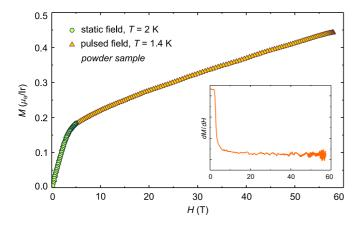
FIG. 4. Field-dependent magnetization measured on a powder sample in static and pulsed fields at T = 2 K and 1.4 K, respectively. The inset shows the derivative of the pulsed-field data.
