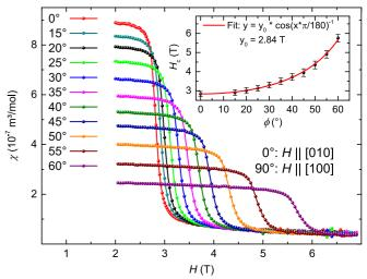
FIG. 5. Field-dependent magnetic susceptibility measured in the fields applied in between the *a* and *b* directions. The transition field  $H_c^{\phi}$  is defined as the midpoint of the steplike decrease in  $\chi$ . The inset shows the angular dependence of  $H_c^{\phi}$  and its cosine fit as explained in the text.
