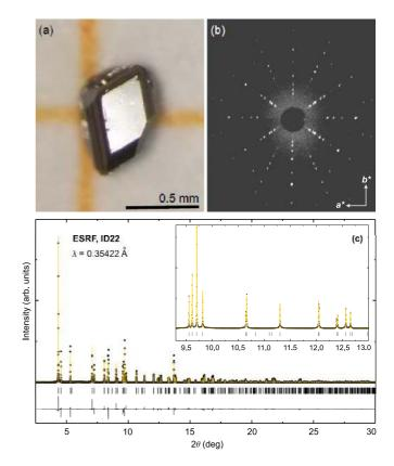
FIG. 1. (a)  $\beta$ -Li<sub>2</sub>IrO<sub>3</sub> single crystal. (b) X-ray Laue-back-reflection-pattern for the beam parallel to [0 0 1]. (c) Rietveld refinement of the synchrotron XRD data: Experimental (dots), calculated (yellow line), and difference patterns (gray line) are shown; the tick marks show the peak positions. The inset magnifies the pattern in the  $2\theta = 9.3-13.0^{\circ}$  range.
