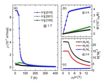
FIG. 2. (a) Temperature dependence of the magnetic susceptibility  $\chi$  measured on an individual single crystal at H = 1 T for three field directions. (b) Field dependence of the magnetization measured along the same directions up to 14 T at 2 K. (c) Anisotropy of the magnetization as a function of field.
